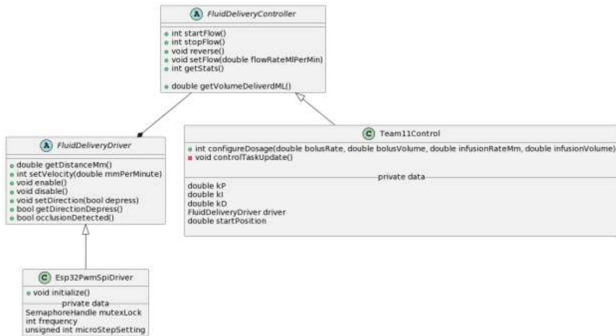
Figure 6. Software Architecture of the Pump Control System
